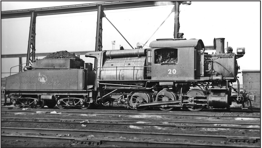
Central Rail Road of New Jersey #20, a 0-6-0 camelback switcher. The fireman froze and the engineer roasted. – Photo, Tom Klinger collection.
