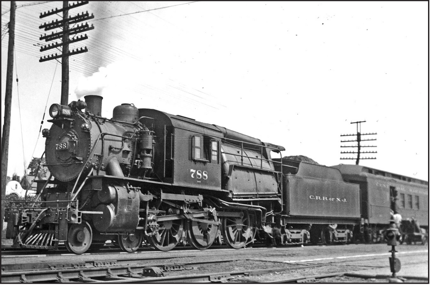
Central Rail Road of New Jersey #788, a 4-6-0 camelback on a passenger train. The wide firebox was needed to burn the region's anthracite coal. – Photo, Tom Klinger Collection.
