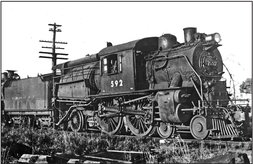
Central Rail Road of New Jersey #592, a 4-4-2 fast passenger camelback engine. Note the railing along the firebox for fireman access. – Photo, Tom Klinger collection.
